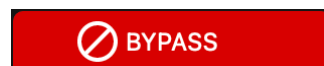
The Bypass button is lit red when the User IR/Factory Cab is bypassed
